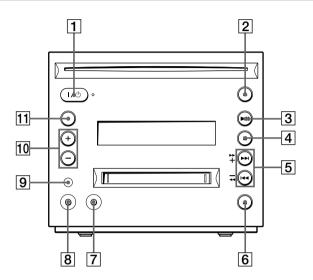
CD SYNC HIGH 7 (19, 51) CD SYNC NORMAL 8 (19) CD 2 (10, 51) FUNCTION 1 (9, 11, 13, 14, 16, 21–37, 44) MD 6 (15, 18, 26) REC/REC IT 8 (20, 21, 24, 26, 44, 51) Remote sensor 9TUNING +/- 5 (36, 37) VOL +/- 10 (40)
